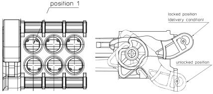
Figure 2-4. 6-pin Power & I/O Connector (Phoenix Contact part)
