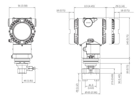
Figure 9 Transmitter with barrel housing – adapter straight (180°) entry connection for sensor E to S
