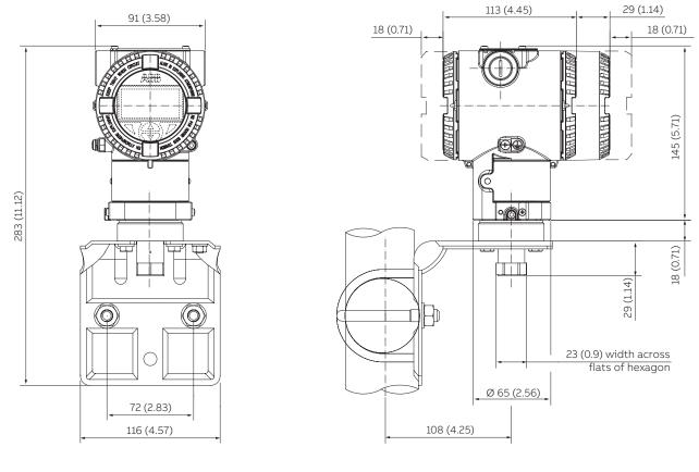
Figure 3 Transmitter with barrel housing – F250C female connection for sensor Z
