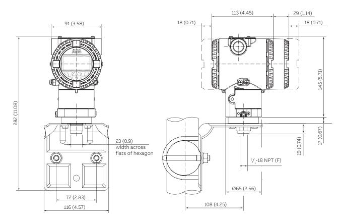
Figure 4 Transmitter with barrel housing – 1/4 in. NPT female connection for sensor Z
