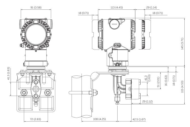
Figure 7 Transmitter with barrel housing – DIN-EN837-1 G 1/2 B connection for sensor E to S
