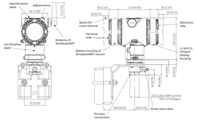
Figure 1 Transmitter with barrel housing –  $\frac{1}{2}$  in. NPT female connection for sensor E to S
