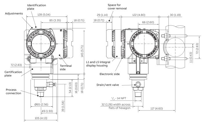
Figure 5 Transmitter with DIN aluminium housing – ½ in. NPT male connection for sensor E to S
